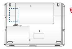
WARNING! Disconnect all the connected peripherals, any telephone or telecommunication lines and power connector (such as external power supply, battery pack, etc.) before installing or removing a memory.
